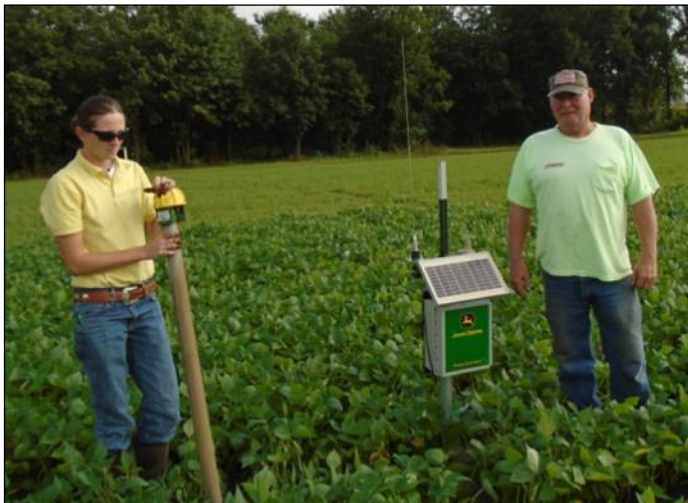
Soil moisture probe installation
