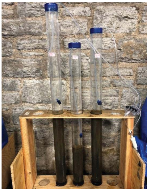
Figure 2. Eagle Lake sediment cores set up in the laboratory for the phosphorus release study.
