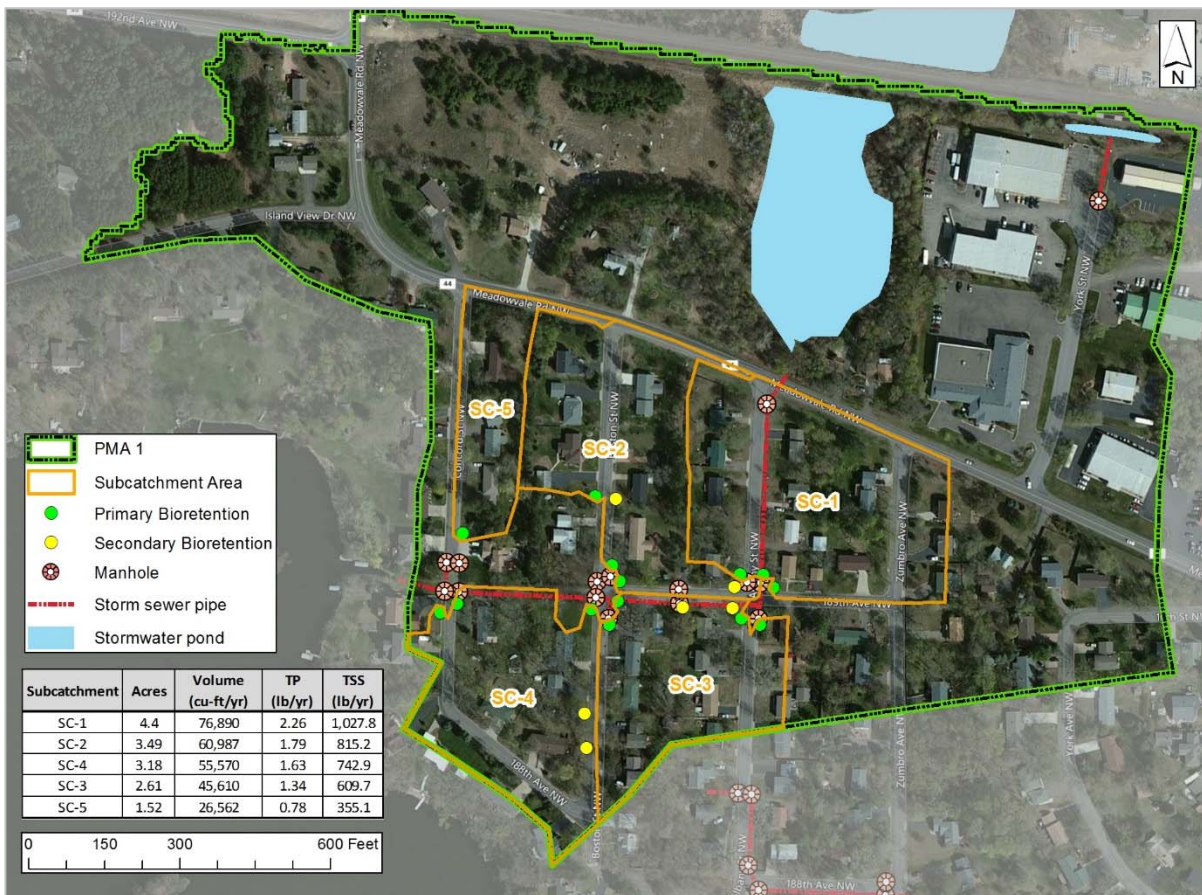
Figure 7: Priority Management Area 1, proposed area for bioretention cells. Map indicates the delineated PMA, delineated subcatchment areas, subcatchment existing loading conditions (sorted highest to lowest), storm sewer routing and proposed primary and secondary bioretention locations.
